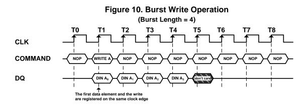
A write burst without the auto precharge function may be interrupted by a subsequent Write, BankPrecharge/PrechargeAll, or Read command before the end of the burst length. An interrupt coming from Write command can occur on any clock cycle following the previous Write command (refer to the following figure).
