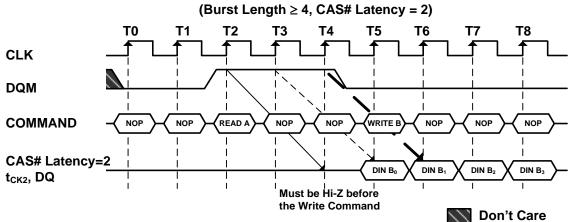
A read burst without the auto precharge function may be interrupted by a BankPrecharge/PrechargeAll command to the same bank. The following figure shows the optimum time that BankPrecharge/PrechargeAll command is issued in different CAS latency.
