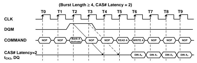
Figure 7. Read to Write Interval
