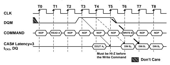
Figure 8. Read to Write Interval
