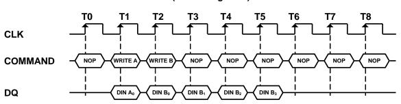
The Read command that interrupts a write burst without auto precharge function should be issued one cycle after the clock edge in which the last data-in element is registered. In order to avoid data contention, input data must be removed from the DQs at least one clock cycle before the first read data appears on the outputs (refer to the following figure). Once the Read command is registered, the data inputs will be ignored and writes will not be executed.
