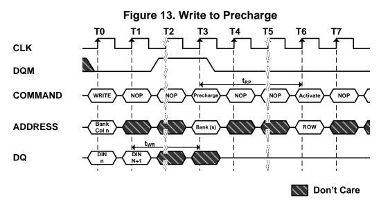
Note: The LDQM/UDQM can remain low in this example if the length of the write burst is 1 or 2.
