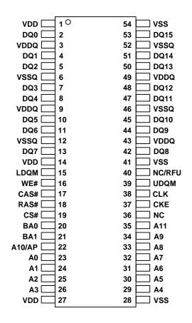
Figure 1.1 Ball Assignment (Top View)
